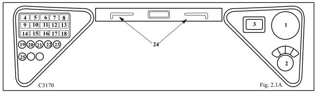
**1. Fuel Gauge:** The fuel gauge indicates the quantity of fuel remaining in the fuel tank.
