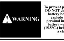
To prevent personal injury DO NOT charge a frozen battery because it can explode and cause personal injury. Let the battery warm to 60°F. (15.5°C.) before putting on a charger.
