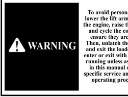
To avoid personal injury, lower the lift arms, shut off the engine, raise the seat bar and cycle the controls to ensure they are locked. Then, unlatch the seat belt and exit the loader. Do not enter or exit with the engine running unless as specified in this manual or under specific service and backhoe operating procedures.
