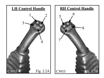
**1. Two Speed Switch (not available on all models):** This switch provides alternate switching. Press to activate Hi-Speed function. Pressing and releasing the switch a second time will return the loader to the Low-Speed function. (See Fig. 2.2A)
